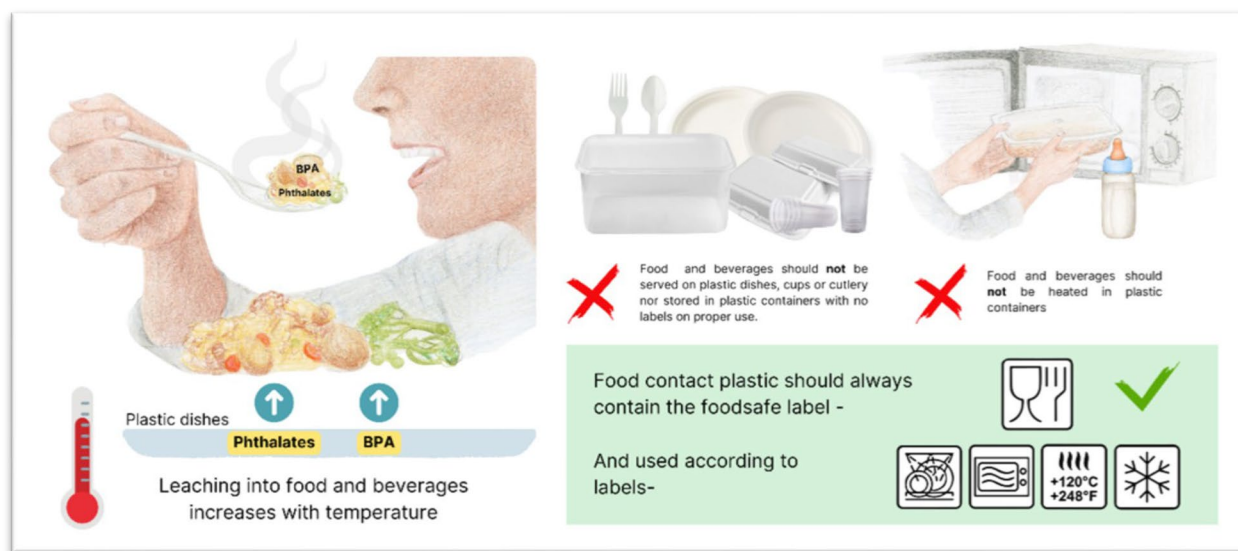
Fig. 5 Leaching of toxic additives from plastic to food and beverages and how to reduce exposure. Citations; Leaching [3, 84, 87, 112–114]; Do's and Don'ts for use of food contact plastic [112]
